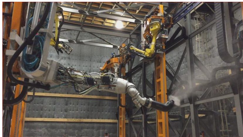
Figure 11 Large Component Painting Automation
